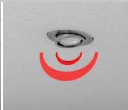
Unwanted sound easily travels through any perforation such as lighting or ducting.
